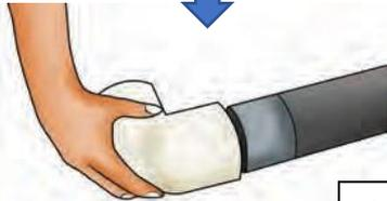
Assemble the edges when the cement solvent is wet
