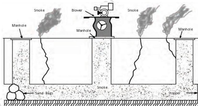
Fig 2.11 Smoke test
