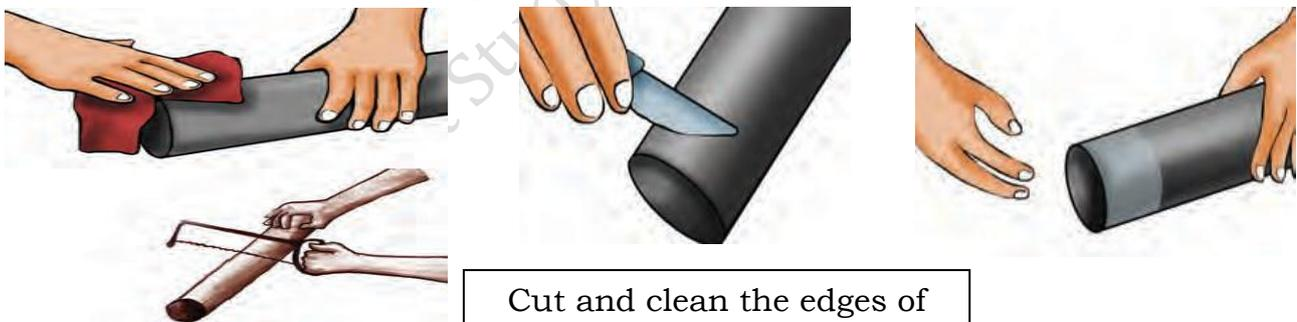
Cut and clean the edges of the pipe
