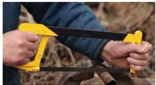
Fig 2.3 Cutting with a hacksaw
