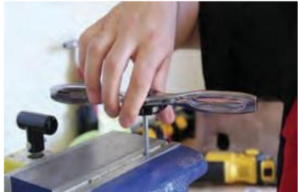
Fig 2.6 Turning steel rod into bolt
