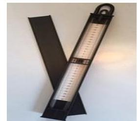
Fig 5.17 Standard U Gauge Manometer
