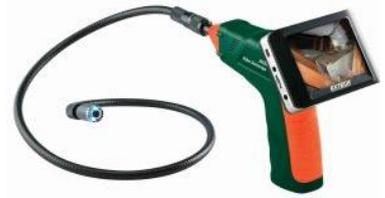
Fig 5.15 Borescope
