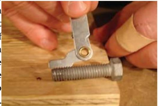
Fig 2.4 Measuring the thread per inch
