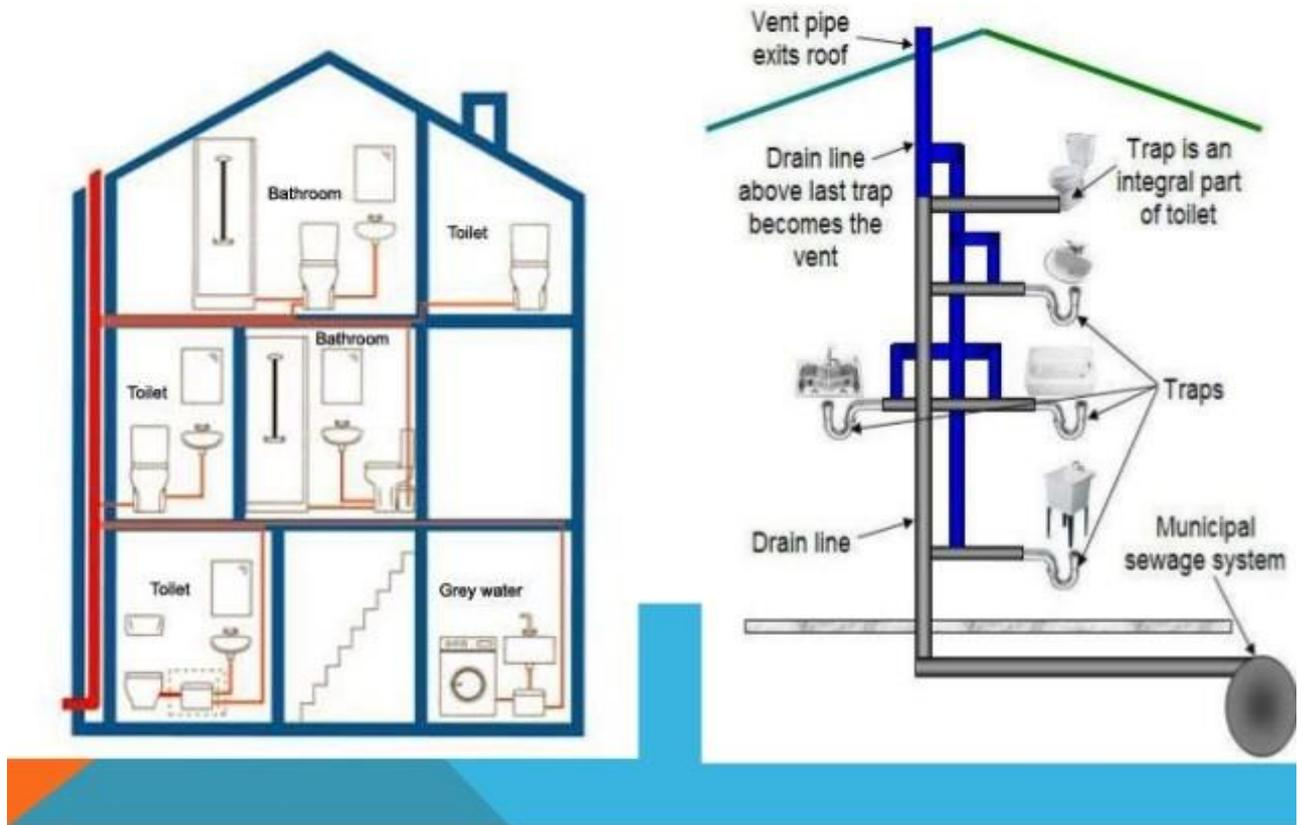
Fig 1.2 Sectional View of building with sanitary system
