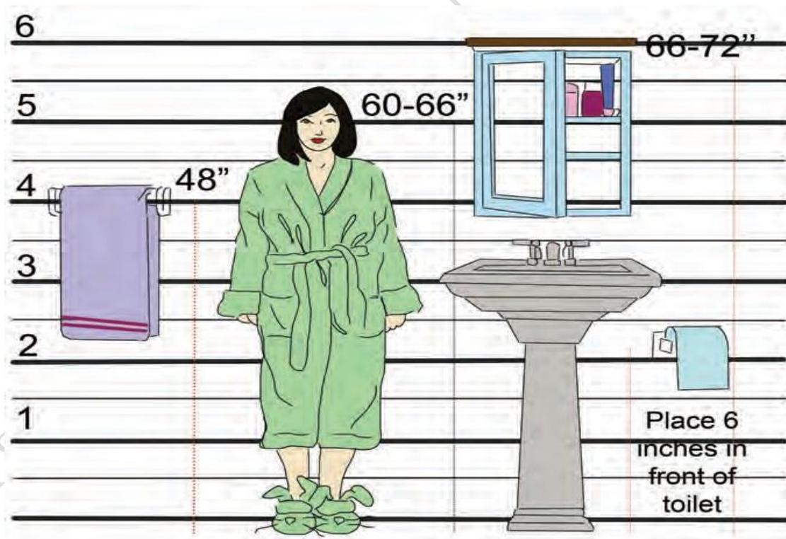
Fig 3.19 Standard height of fixtures in bathroom in inches
