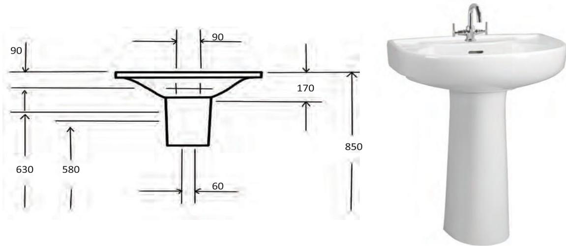
Fig 3.18 Installing a pedestal washbasin with a standard
