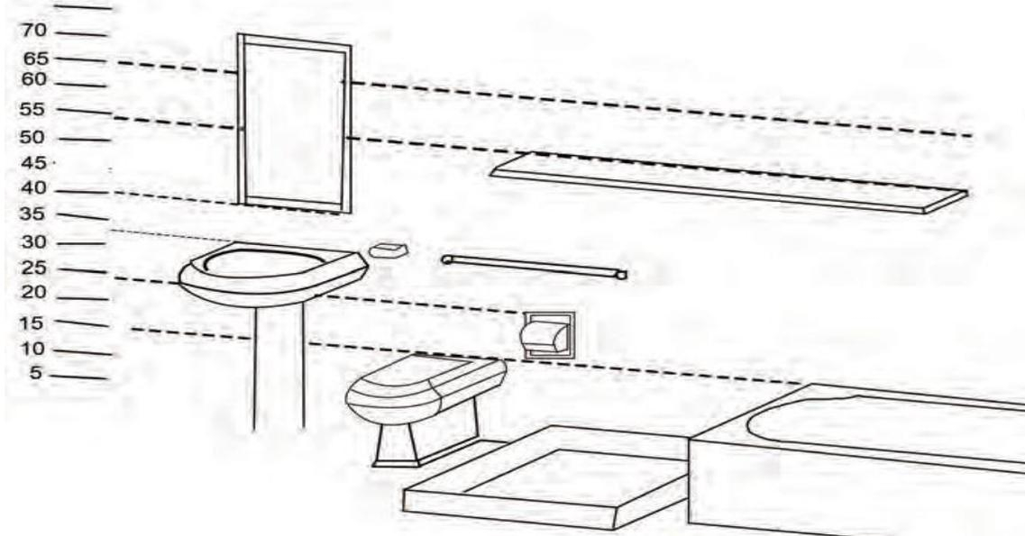
Fig 3.17 Standard height of sanitary fixtures (*Dimensions are in inches*)
