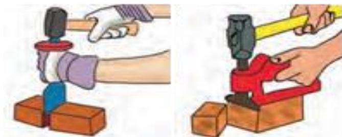
Fig 1.10 Cutting of bricks using chisel
