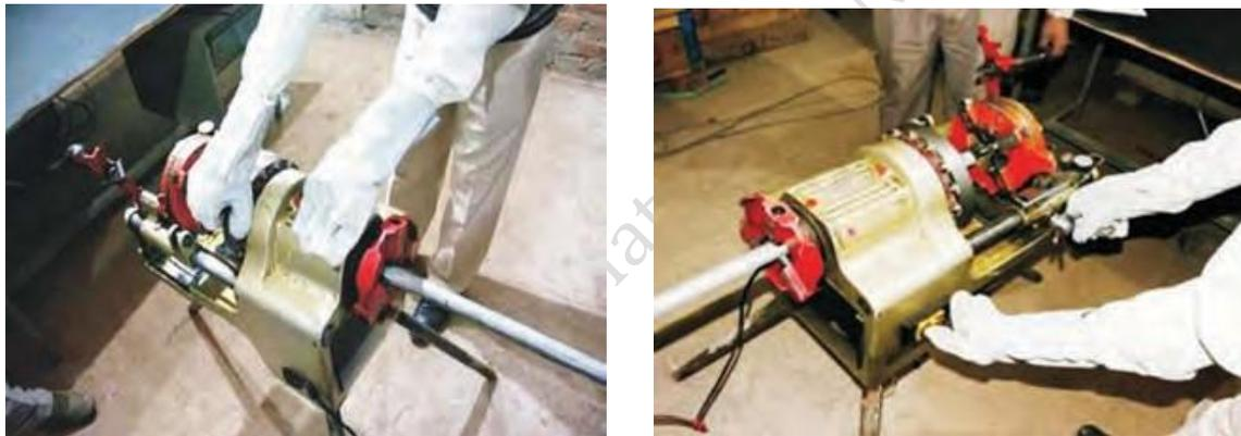
Fig 2.9 Pipe Threading using Pipe Threading machine
