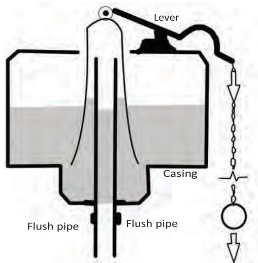
Fig 3.13 Bell Flushing Cistern
