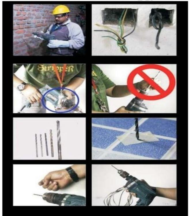
Fig 1.4 Precautions to be taken while using a drill
