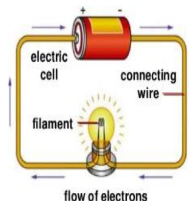
Fig 5.1 Flow of electricity
